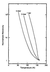
Figure 3: Normalised resistivity versus termperature curves for (TMTTF)<sub>2</sub>SbF<sub>6</sub> at 1 bar, 3 and 5 kbar.
