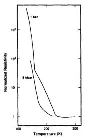
Figure 2: Normalised resistivity versus termperature curves for (TMTTF)<sub>2</sub>ReO<sub>4</sub> at ambient pressure and 5 kbar.
