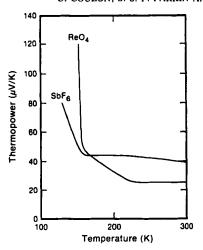
Figure 1: Thermopower versus temperature curves for (TMTTF)<sub>2</sub>ReO<sub>4</sub> and (TMTTF)<sub>2</sub>SbF<sub>6</sub>.
